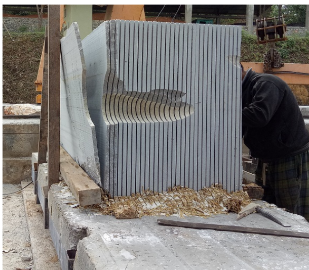
Gang saw machine cut slab
